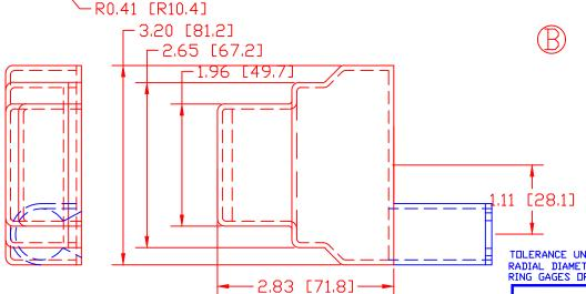
TOLERANCE UNLESS OTHERWISE SPECIFIED: ±.030"/±0.8mm RADIAL DIAMETERS TO BE MEASURED OVER MANDRELS, RING GAGES OR PIN GAGES OF SUITABLE SIZE
