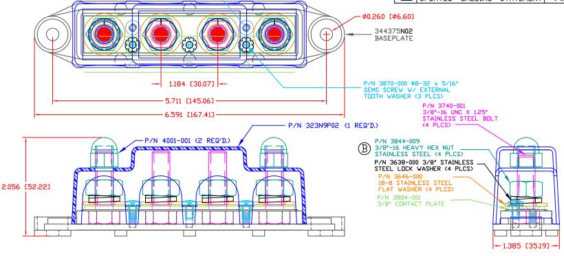
MATERIAL PART NO: MATERIAL: VENDOR PART NO: SPECIFIC GRAVITY: MELTING TEMP: U.L. RATING: 7111210502 GLASS FILLED NYLON HYLON N2015 HL NAT 1.23 515 F [268 C] UL 94 HB
